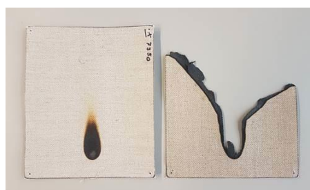
Figure 2. Coated textile with commercial FR after ISO 15025. Left: optimized FR, right: no FR.
