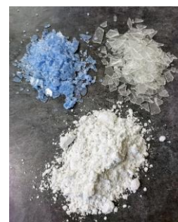
Figure 2 Frits (above) milled to Powder
